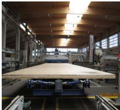
CLT element ready for cutting and joining
