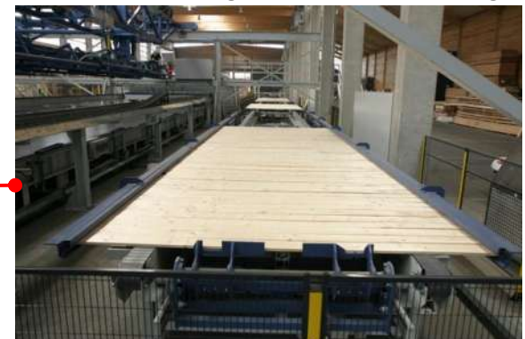
cross layers composing & compressing
