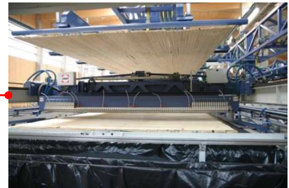
adhesive application next layer stand-by
